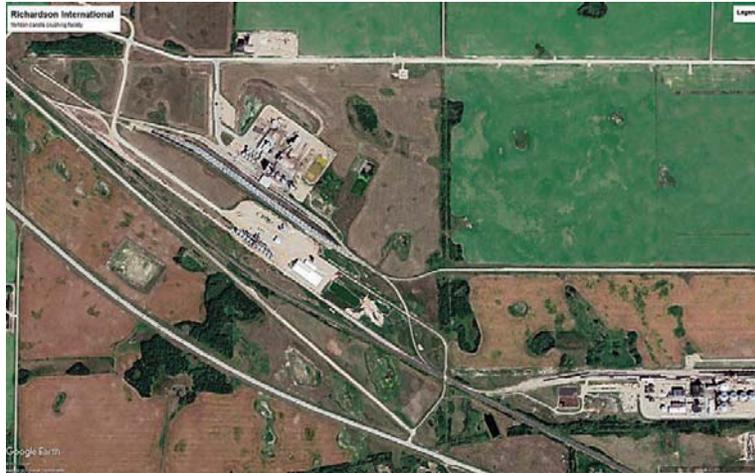
This Google Earth image shows the Richardson International canola crush facility at Yorkton on the left side of the map. To the right is the area where the triple loop track will be installed. The rail line going northwest/southeast is the Canadian Pacific mainline. The line going straight east connects to the CN rail network. The facility on the lower right is the Louis Dreyfus Company canola crush plant.
